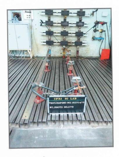
Mounting arrangement (Before test)
